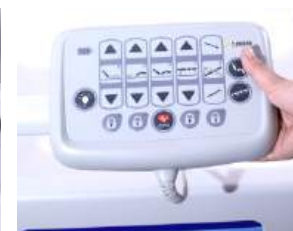
Locking Mechanism: All positions can be locked individually by ACP except the auto CPR.
